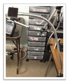
Gooseneck Mounting System – Allows for convenient positioning. Now you can position a switch anywhere you'd like. Equipped with a flexible, extra stiff gooseneck, you can attach it to a table or wheelchair using a unique clamp.
