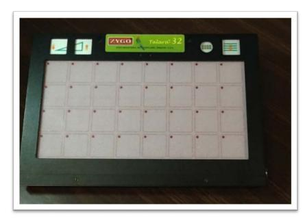
Zygo Talara 32 - The Talara-32 is a simple communication aid that records human voice and other sounds for playback. It is an electronic communication device with *four levels*, direct and switch scanning access and flexible size key patterns making it easily customizable for both children and adults with wide ranging abilities and needs.
