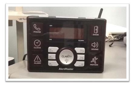
Clarity Alertmaster A10 Signaling system – The Clarity is a complete alerting system that alerts you to the telephone, alarm clock and doorbell by light and vibration. The system also has different flashing patterns so you can distinguish between the door, telephone, alarm clock, or one of the other optional transmitters that can be added to this system.
