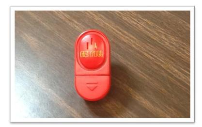
**EZ Fill** - Device that buzzes to indicate that a liquid has reached about 1 inch from the top of a container.
