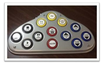
Jumbo Universal Remote Control- This universal remote allows user to easily see and push buttons to control TV, VCR, DVD, Cable and Satellite receivers. The large buttons are very sensitive to touch and have different colors for different group functions. If you cannot hit the buttons, jacks on the back allow you to plug in your special ability switches. Easy to program, easy to use.
