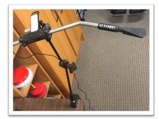
**Flex Switch** – Single switch operated by bending the flexible rubber tip, can be mounted on a wheelchair or table mount.
