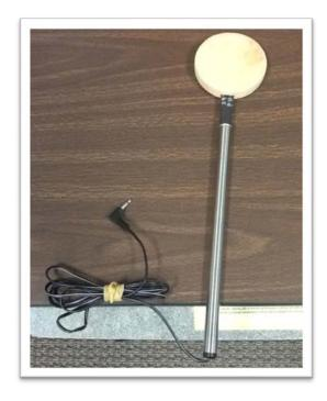
**Leaf Switch-** Activated by pressing lightly against the leaf in one direction. Comes with a removable 3" round foam pad. Tactile and auditory feedback. (Requires mounting).
