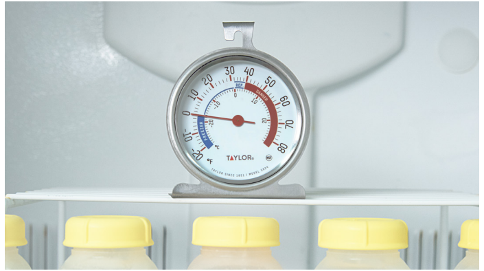
Appliance thermometer showing the freezer temperature is at 0 °F (-18 °C).
