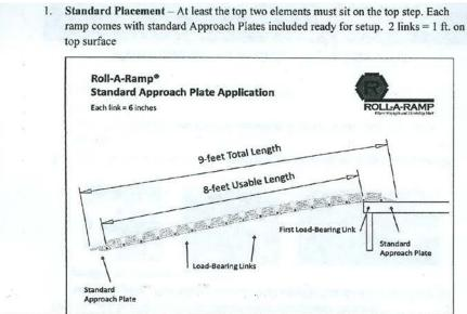
Be sure to place the <u>Upper End</u> of the Ramp on the top step. **It is clearly marked.** The links on the upper end have a 1° camber, while the links on the lower end have a 0° camber.
